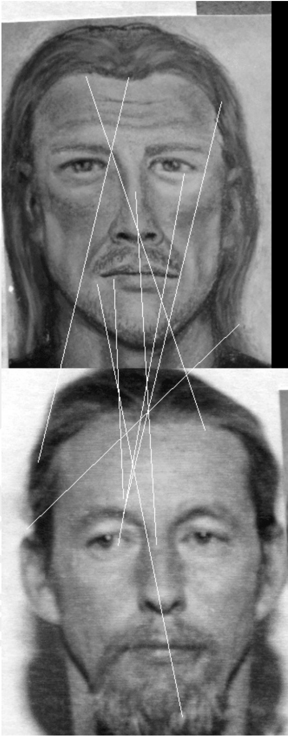
Figure 2.5: An example of forensic sketch matching. The lines show the corresponding features, as depicted by SURF in between the sketch and photo
