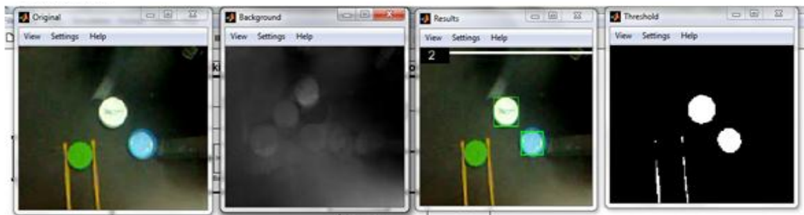
Fig. 7 Output of Background Estimation Method (Multiple Object) a) Actual Image, b) Estimated Background, c) Final Output d) Binary Image after Background Subtraction,
