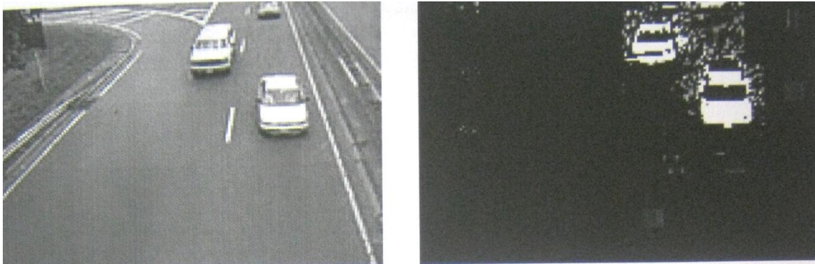
Fig. 10 Output for Light Object without Correlation Actual Image and Masked Contrast Image for Frame No. 33
