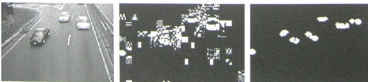
Fig. 12 Output for Dark Object without Correlation Actual Image, Masked Contrast Image and Binary Image for Frame No. 68
