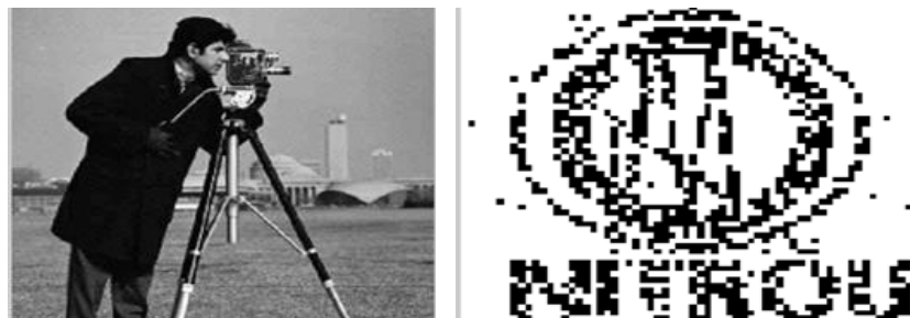
Fig- 7.17 Results after jpeg compression with a multiplication factor 2, and the extracted watermark
