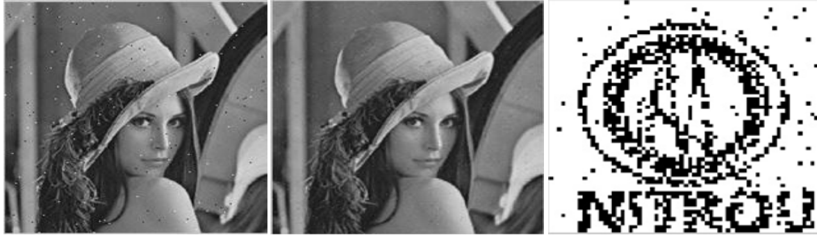
Fig- 7.6 Results of adding impulse noise , then median filtering and the extracted watermark
