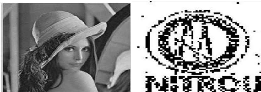
Fig- 7.8 Results after jpeg compression with a multiplication factor 2, and the extracted image
