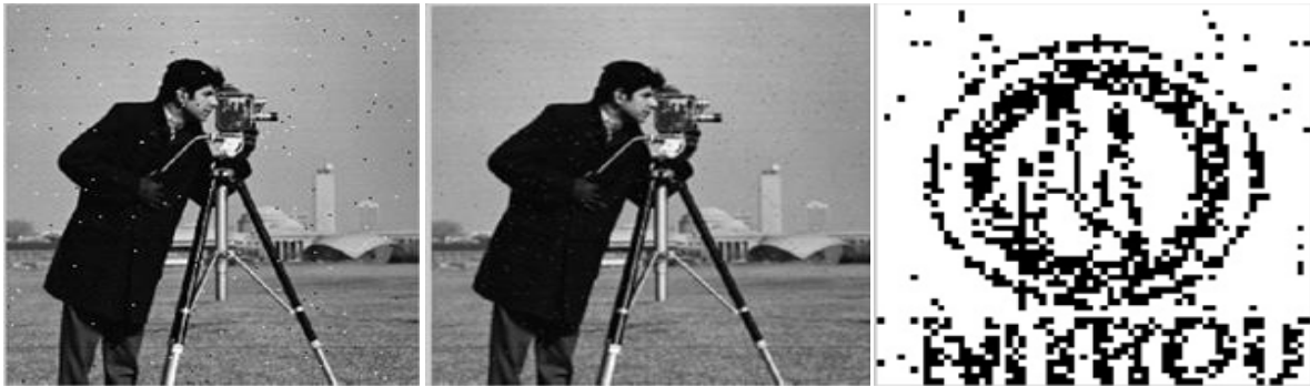
Fig- 7.15 Results of adding impulse noise to the watermarked Image, than doing median filtering operation and the extracted watermark
