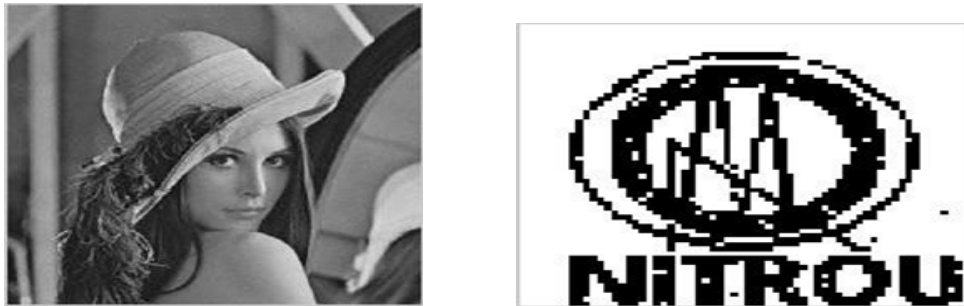
Fig- 7.7 Results after jpeg compression with a multiplication factor 1, and the extracted watermark
