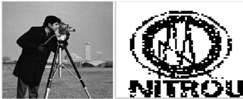
Fig- 7.16 Results after jpeg compression with a multiplication factor 1, and the extracted watermark
