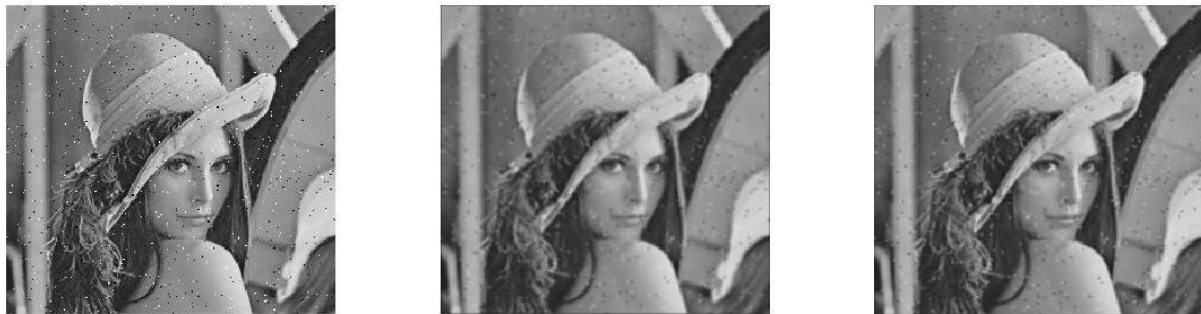
(a) Noisy image (b) Using weighted mean filter (c) Using Arithmetic mean Filter
