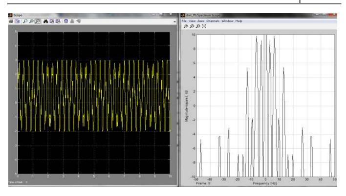
Figure 13: Composite input signal and its frequency response
