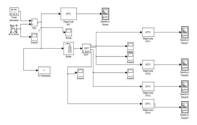
Figure 12: Model based design for Wavelet packet decomposition in Simulink
