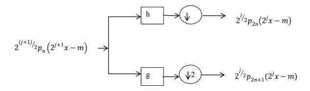
*Figure 8: Wavelet packet decomposition by two-channel filter bank.*[2]
