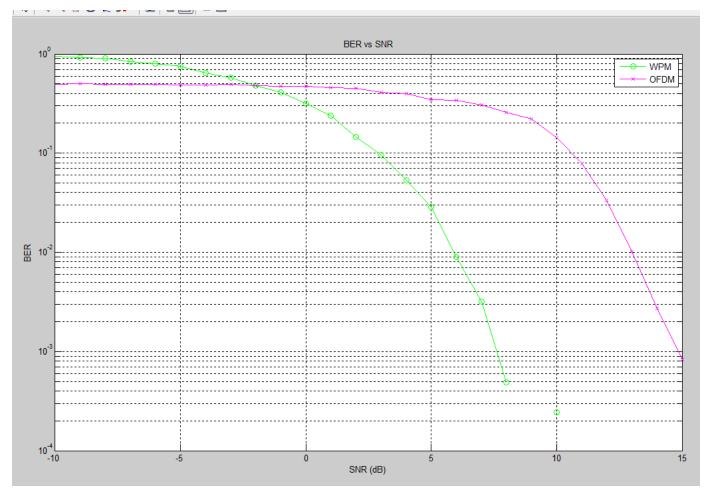
Figure 20: BER vs. SNR plot for comparison of performance of OFDM and WPM
