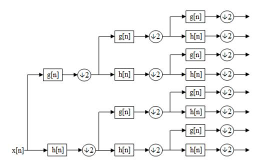
Figure 7: Wavelet Packets of 3 levels of decomposition of signal x[n] [3]
