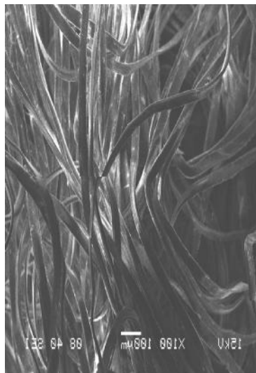
FIG 6: SEM images of sample at 50 0 C,0.02M Na 2 CO 3 ,35 minutes
