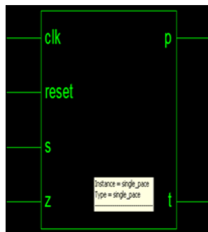
FIG. 3.3 RTL schematic of Single Chamber Pacemaker
