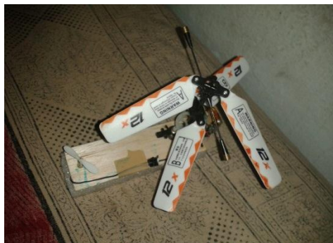
Fig.2.1 Fabricated final model of coaxial micro helicopter.
