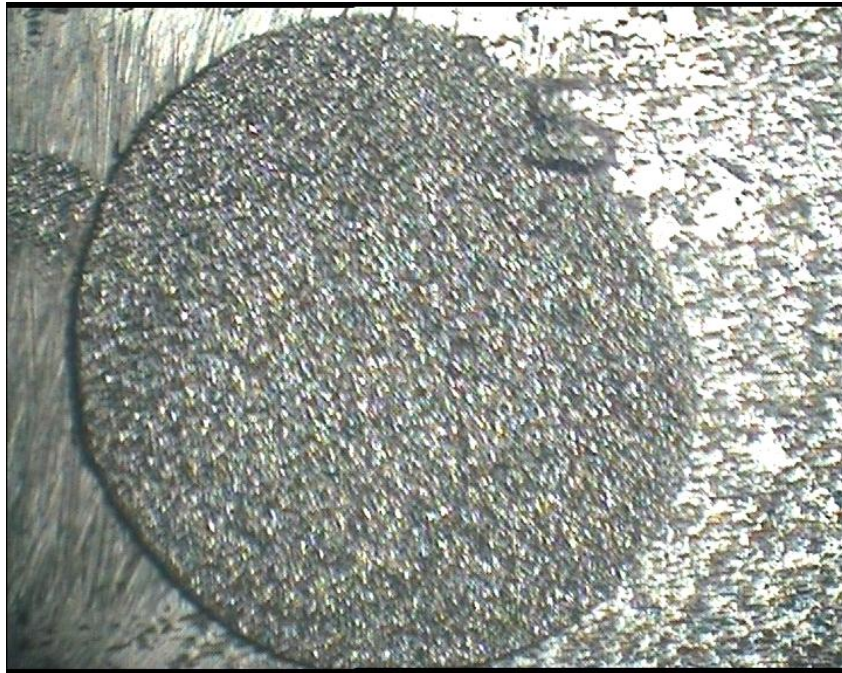
EDM machined surface (Sample No. 5)
