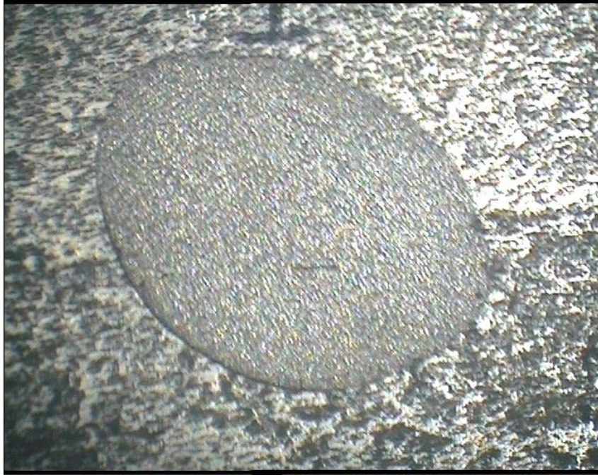
EDM machined surface (Sample No. 1)
