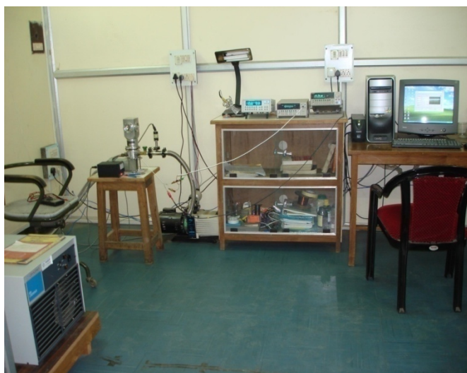
Fig.7: FOUR PROBE SETUP FOR RESISTANCE MEASUREMENT
