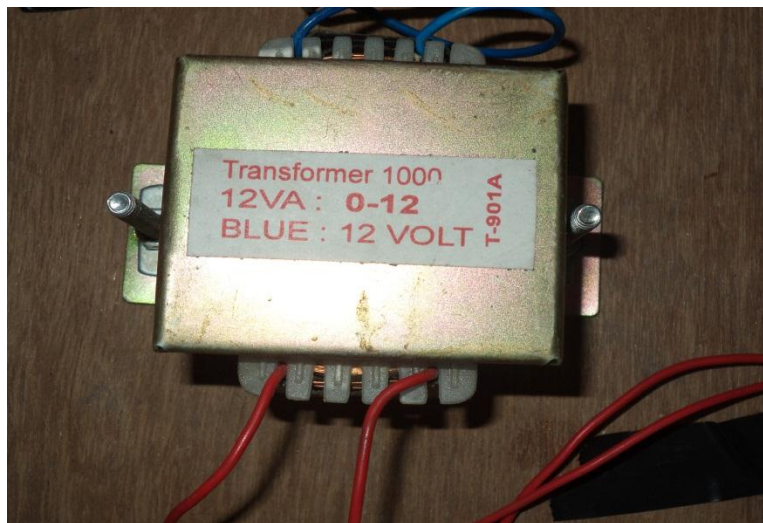
Figure 8 : Step Down Transformer
