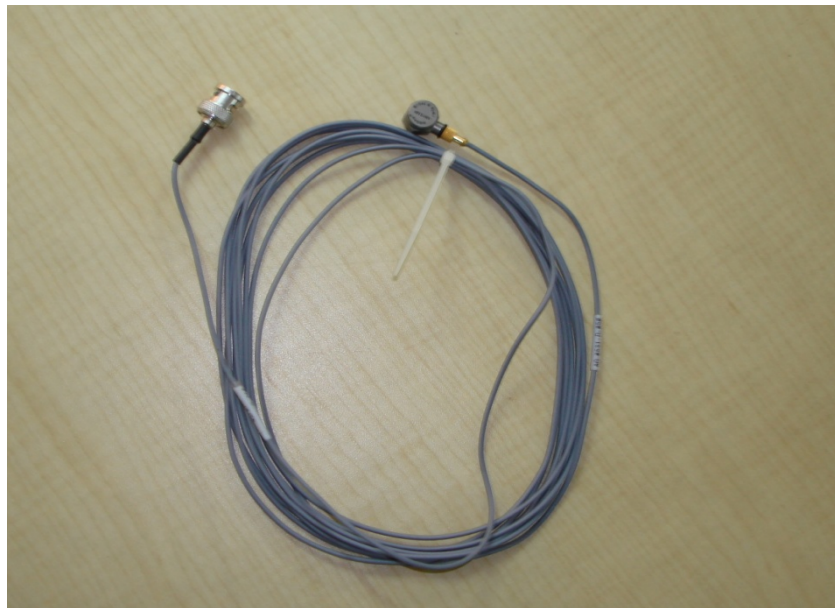
Figure 7.2.3 Vibration Pick-up or Accelerometer
