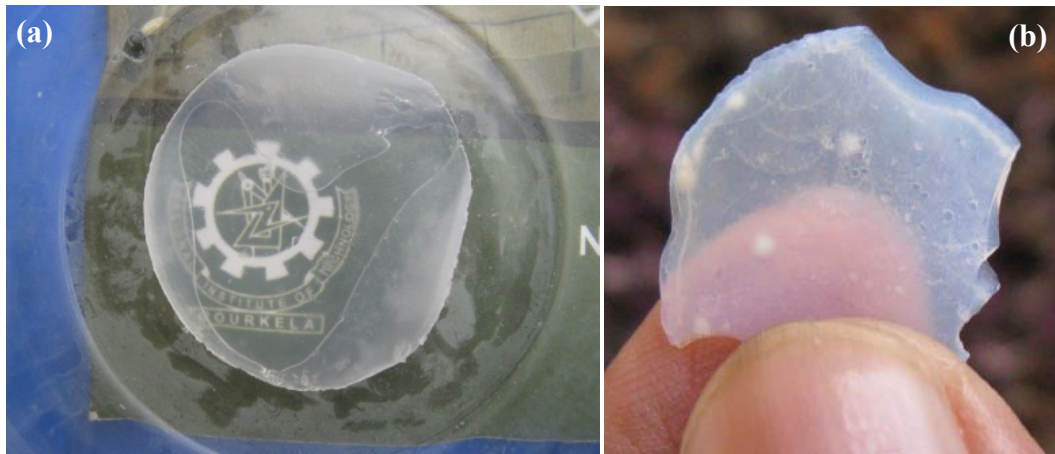
Fig. 4.55 Photographs of silica aerogel (a) strengthened by TEOS, (b) dried monolithic translucent piece.
