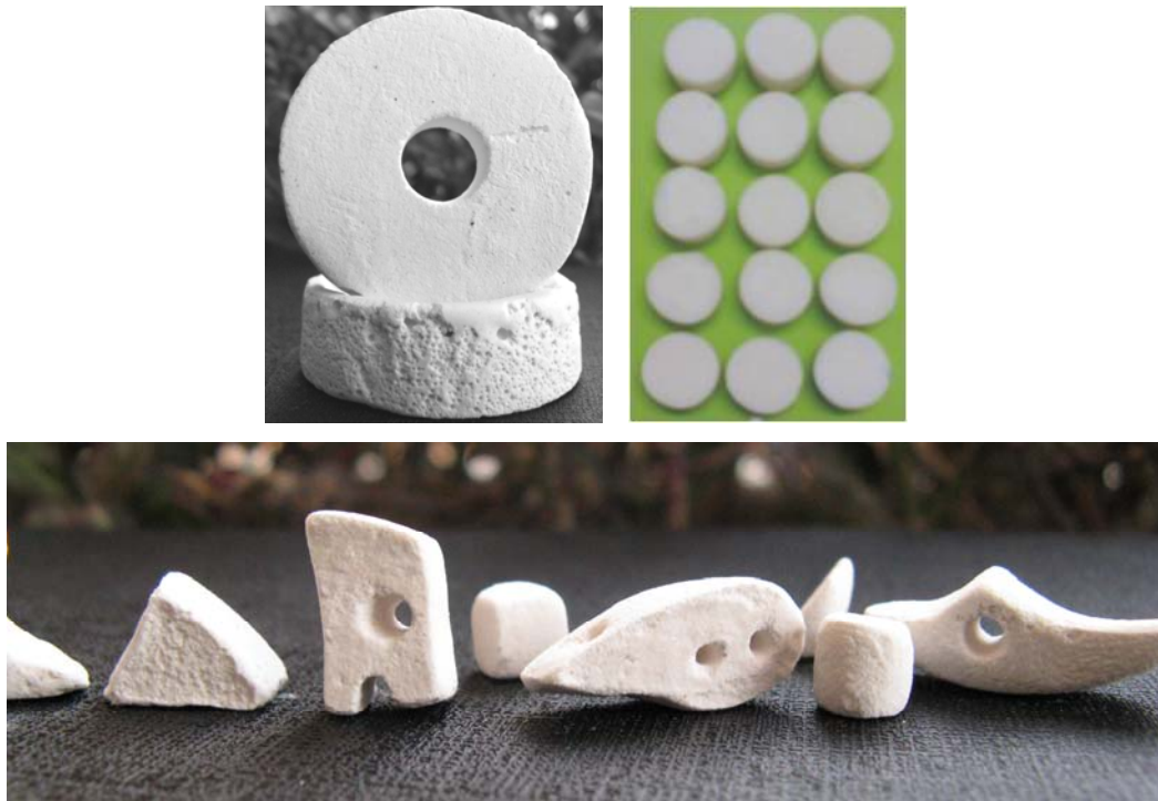
Fig. 4.37 Different sintered shapes prepared by machining gelcasted ingot.
