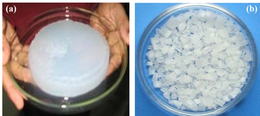
Fig. 3.2 Silica hydrogel (a) and Dried Silica Gel (b).
