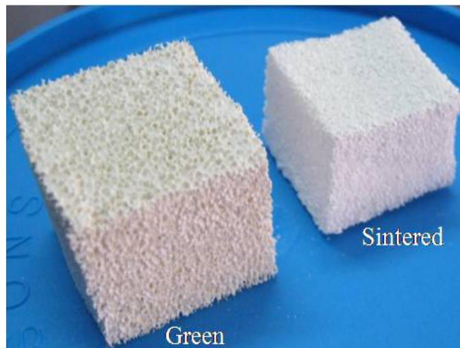
Fig. 4.23 SG-slurry green and sintered sponge cubes.
