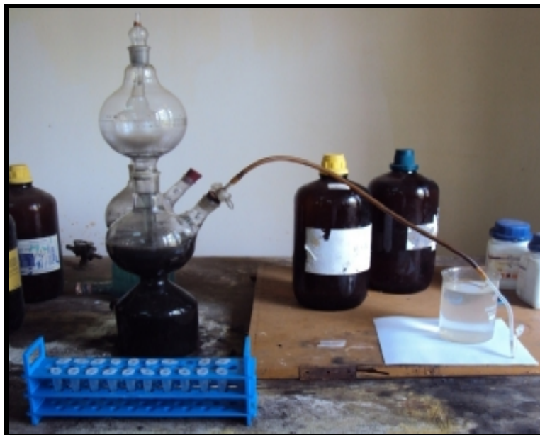
Fig 7. Set-up for the determination of mercury bioaccumulation in mer negative isolates by H 2 S assay
