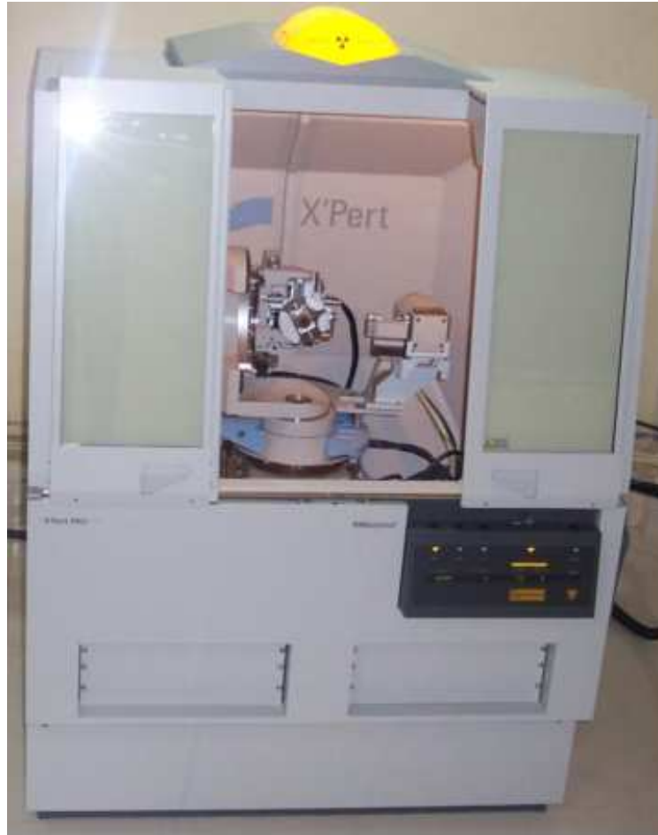
Fig. A.10: Panalytical MRD System for Bulk Texture and Residual Stress Measurement
