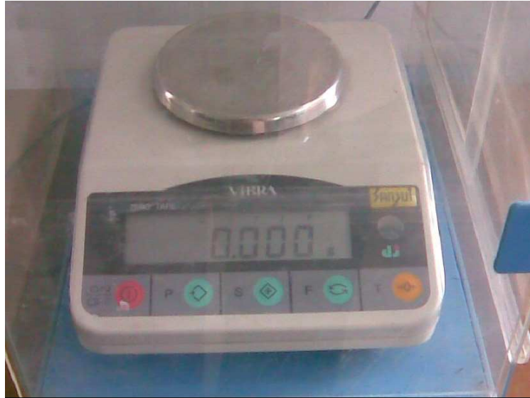
Fig. A.5: Electronic Balance Brand:SHINKO DENSHI Co. LTD, JAPAN, Model: DJ 300S Capacity: 300 gram Accuracy: 0.001 gram
