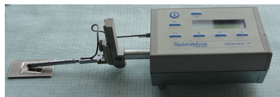
Fig. A.6: Talysurf Surface Roughness Analyser Brand : Taylor Hobson, Model : Surtronic 3 +
