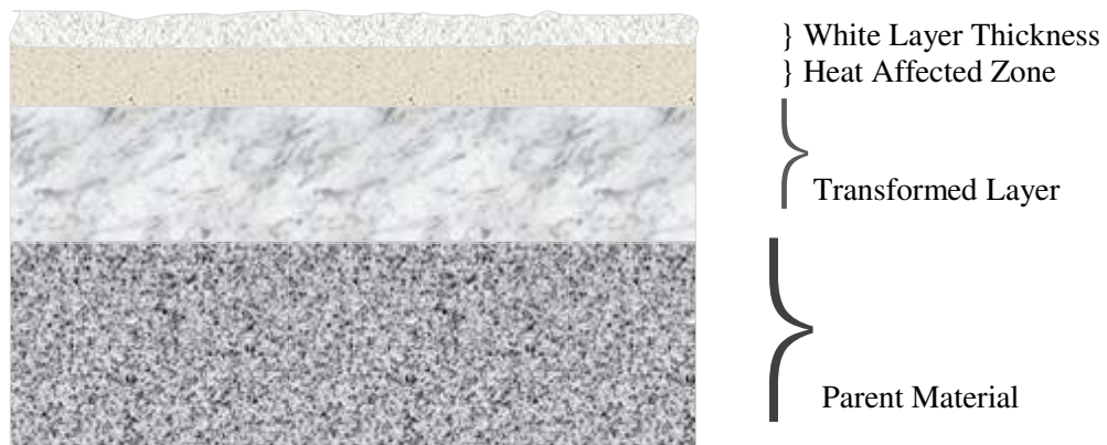
Fig. 2.1: Surface layers in EDMed workpiece
