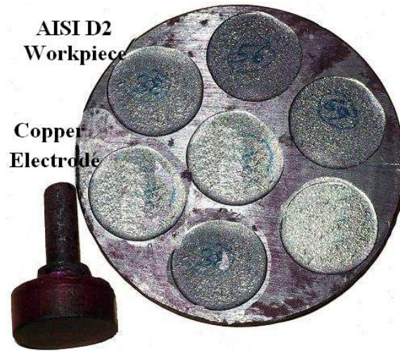
Fig. A.2: Copper Electrode and AISI D2 workpiece for MRR, TWR and OC
