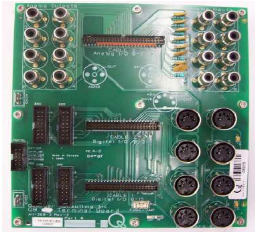
Fig. 3.12 Q8 Terminal board
