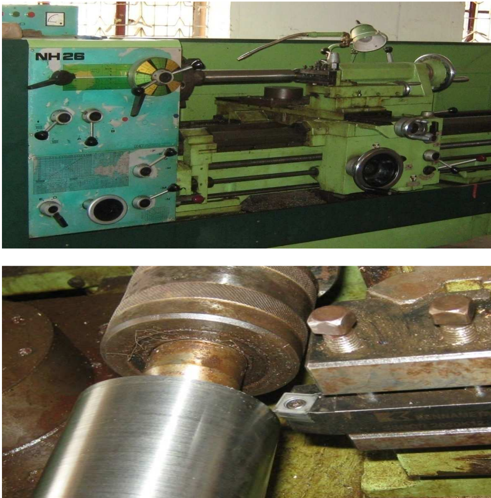
Figure 3.6 Photographs of Experimental Setup for Turning of AISI 316 grade austenitic stainless steel.
