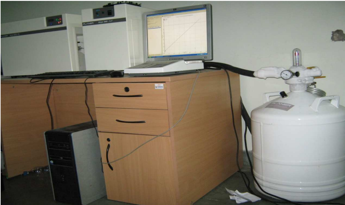
Figure 3.2 Experimental set up for cryogenic treatment
