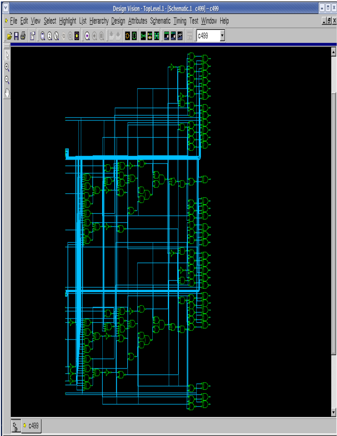
Fig.5.2 Optimized gate level netlist for C499
