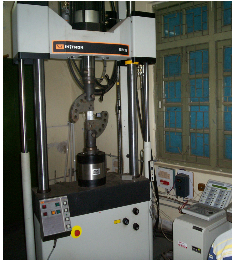
Fig. 3.5 – INSTRON 8502 dynamic testing machine
