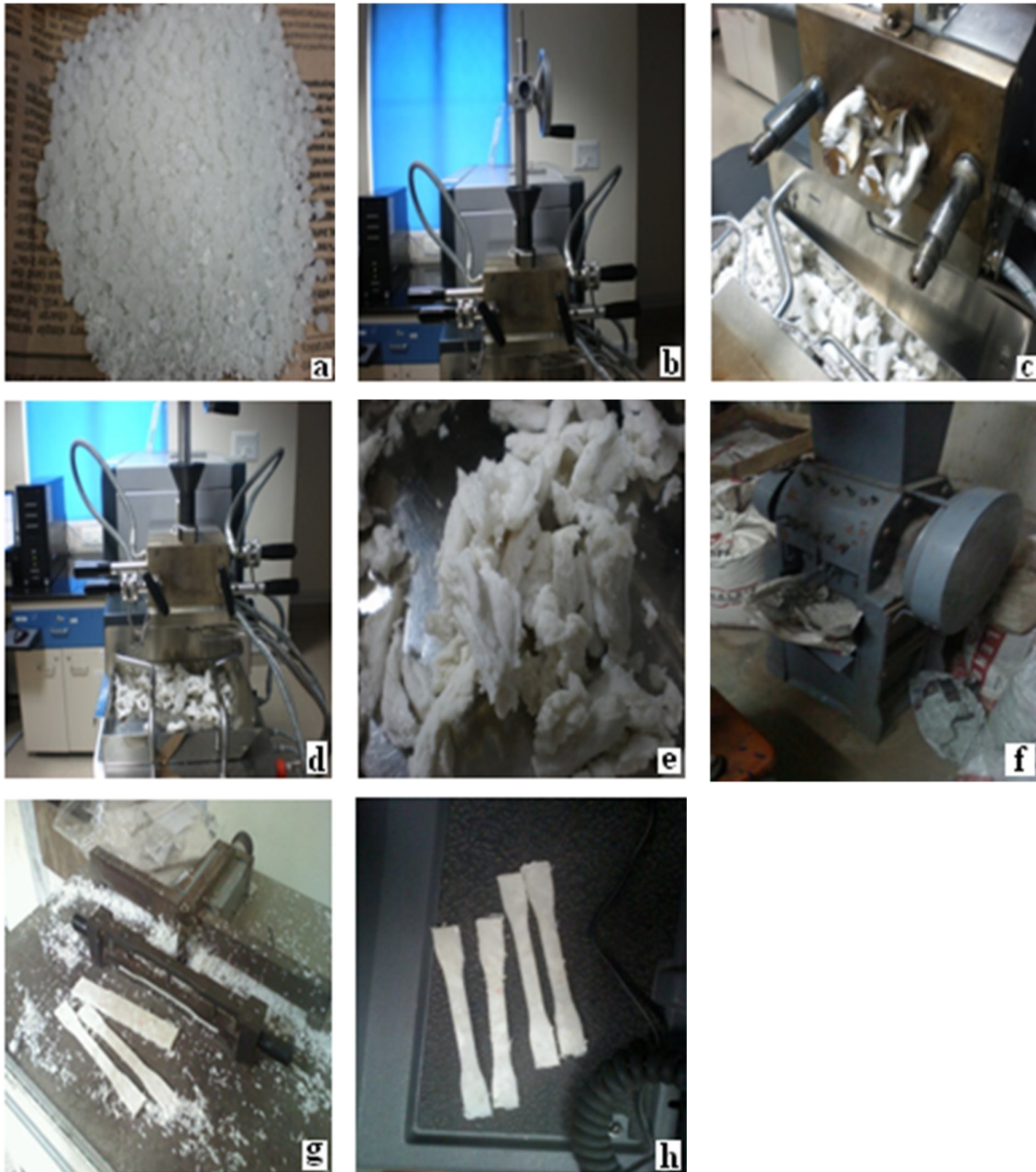
Figure 4.5 Composite preparation through compression molding route: (a) hand mixed HAP and polymer granules, (b-d) mixing in twin screw extruder, (e) mixed composite after mixing in the extruder (f) Grinding Machine (g) contour cutter (h) final shapes of the samples
