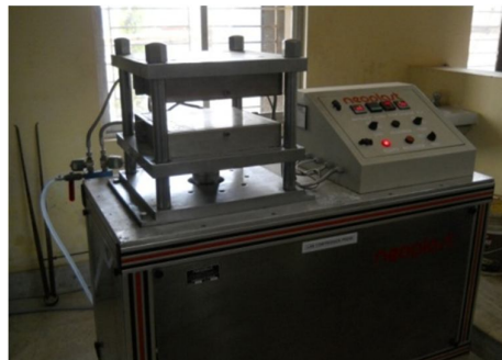
Figure 4.4 NEOPLAST hydraulic press (Compression molding machine) AN INVESTIGATION ON CHARACTERIZATION OF BIO-COMPOSITES
