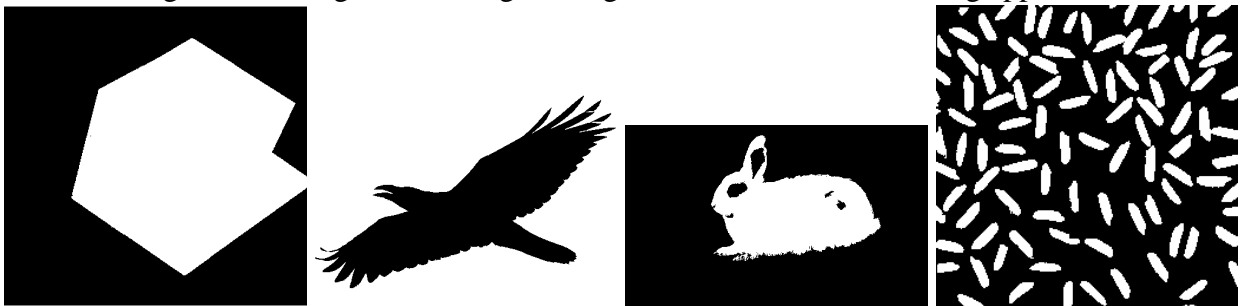
Figure 6.13: Segmented images using Otsu's Global Thresholding approach
