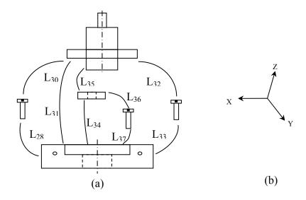
Figure 5.11 (a): Liaison graph model of electromotor subassembly; (b): Directions for assembly or disassembly
