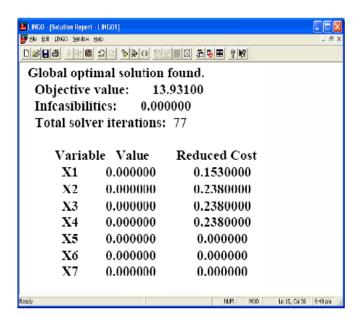
Figure 6.9 Solution report of the LP using LINGO
