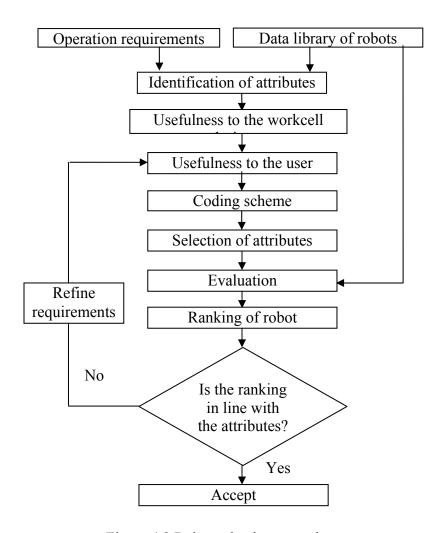
Figure 4.2 Robot selection procedures
