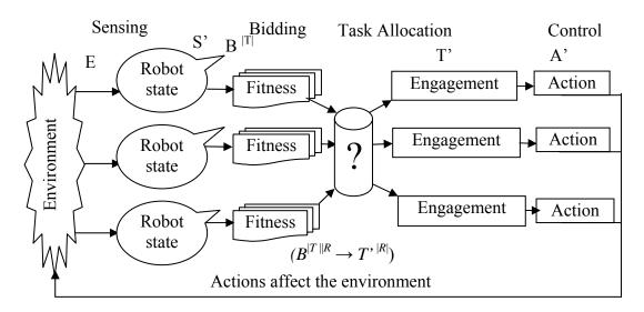
Figure 3.4 Reducing the dimensionality of multi-robot coordination
