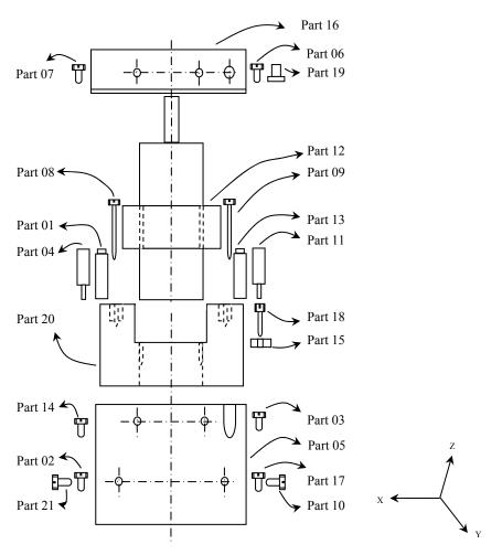
Figure 5.8 Exploded view of a drive assembly
