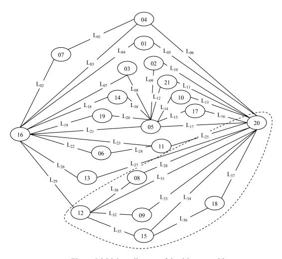
Figure 5.9 Liaison diagram of the drive assembly
