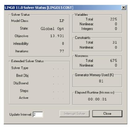
Figure 6.8 Results of the LP using LINGO
