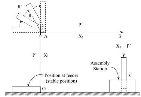
\*P' is Prismatic motion and R' is revolute motion needed during the Task
