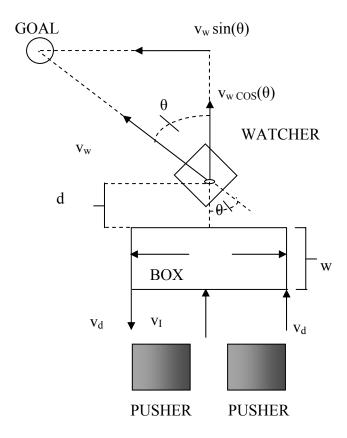
Figure 2.3 The model for deriving the pushing velocities for moving the box along the desired trajectory
