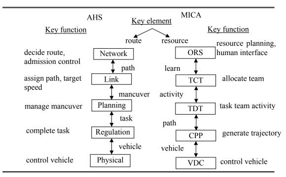
Figure 2.9 The AHS and MICA hierarchies with their key elements and functions
