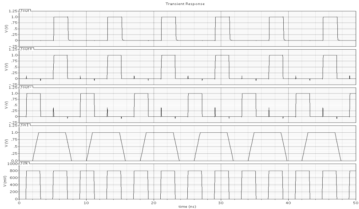
Figure 4.9 Transient Analysis of the comparator.
