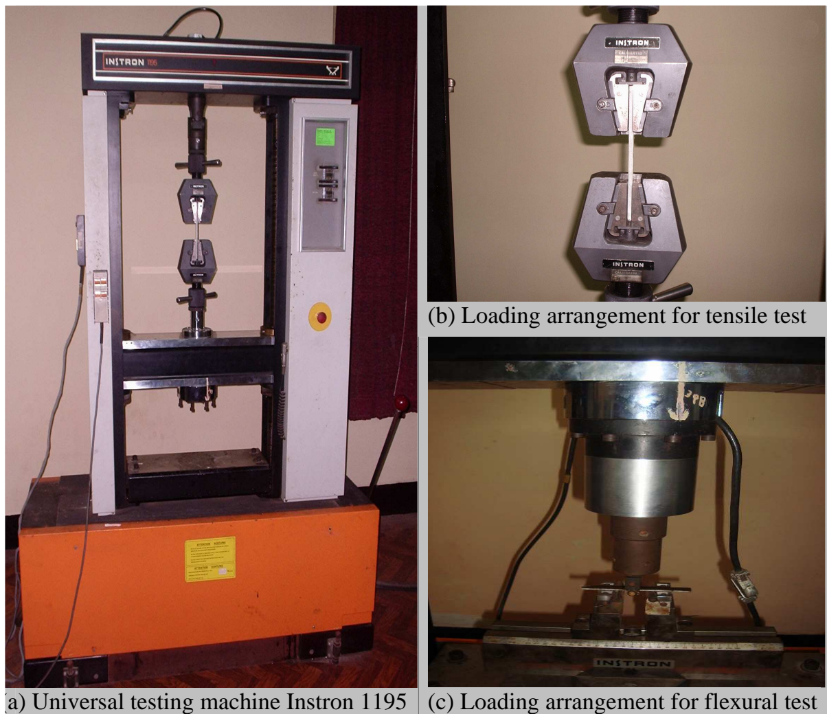
Figure 3.2 Universal testing machine (Instron 1195) and loading arrangement for tensile and flexural tests
