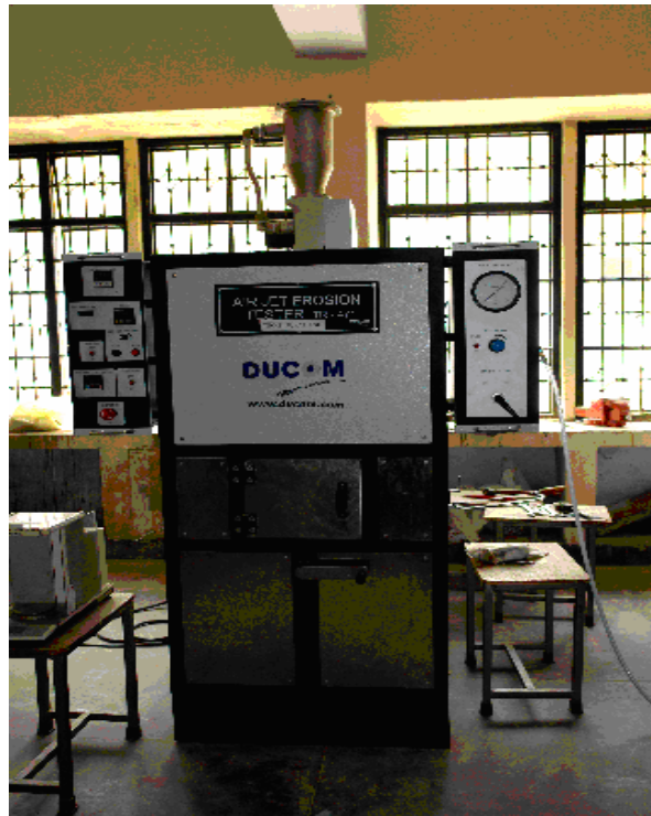
Figure 3.5 Solid particle erosion test set up
