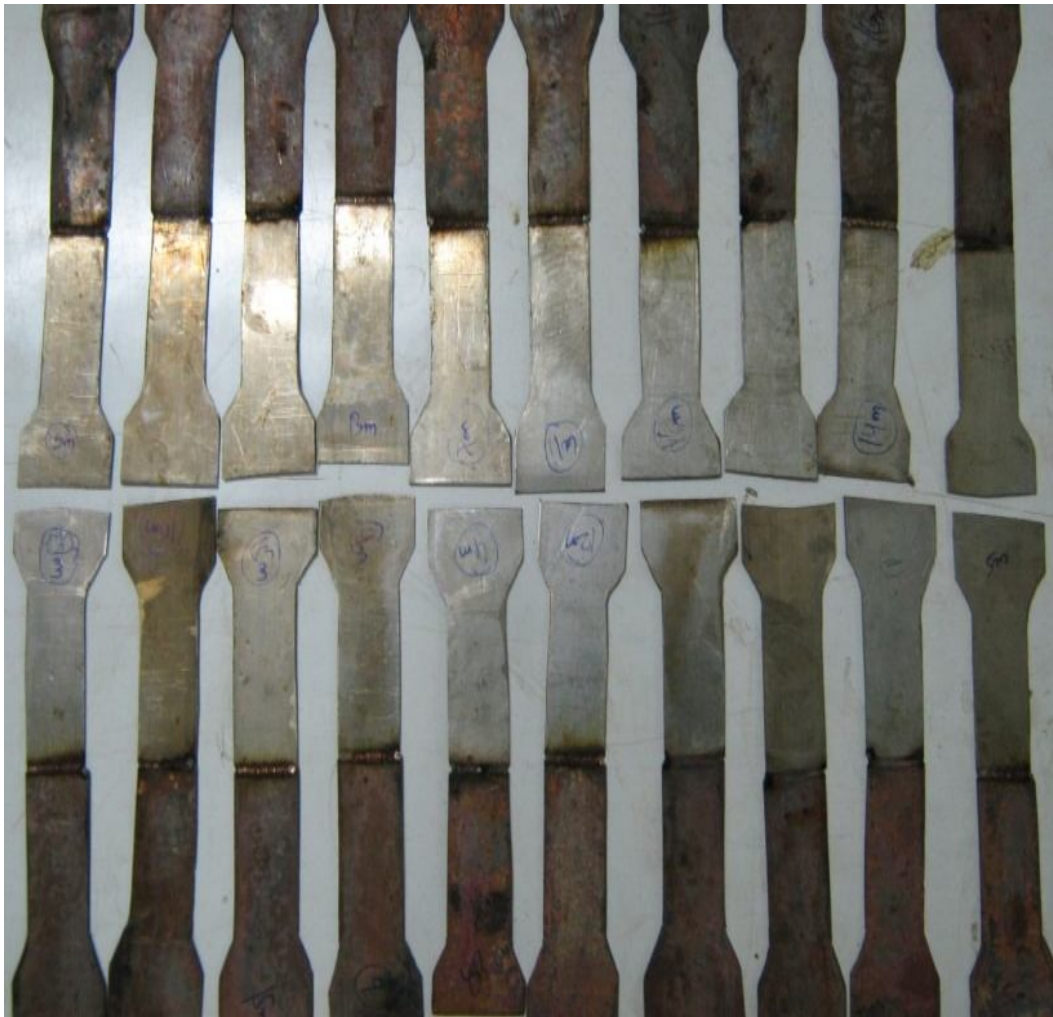
Figure 9 workpiece after welding
