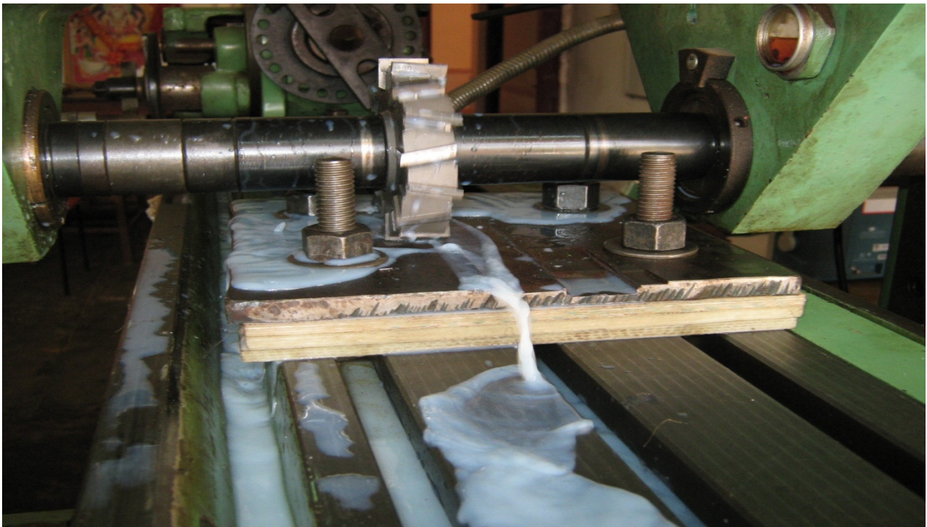
Fig 7.4 Three layers of Glass fiber polyester bolted to the slotted table milling machine
