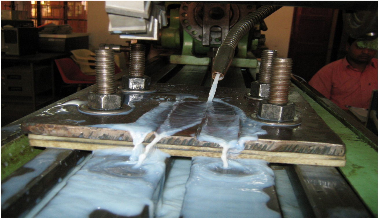
Fig 7.9 Six layered sandwich plates of Glass fiber epoxy and polyester bolted to the slotted table
