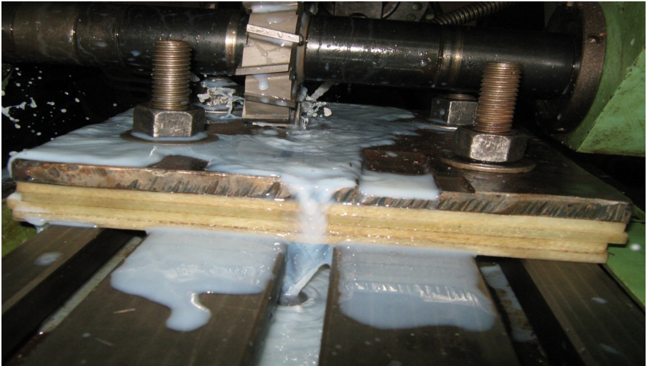
Fig 7.5 Four layers of Glass fiber epoxy bolted to the slotted table milling machine
