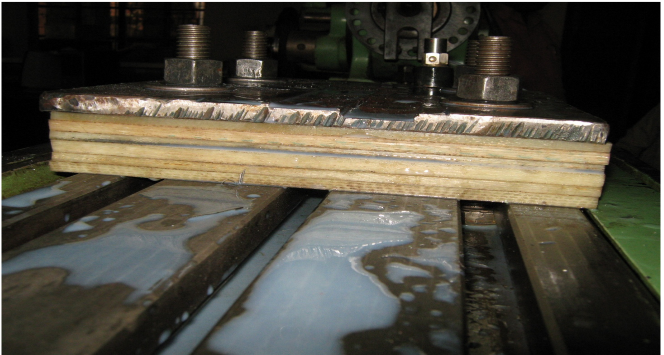
Fig 7.7 Ten layered sandwich plates of Glass fiber epoxy and polyester bolted to the slotted table
