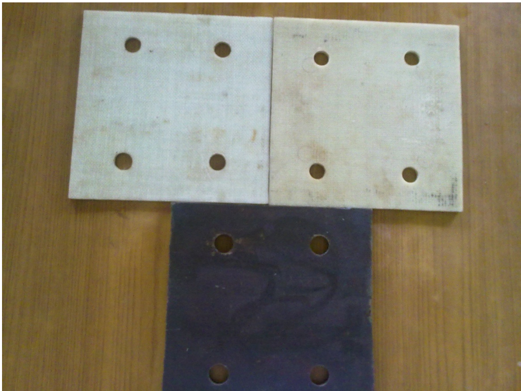
Fig 7.1 Glass fiber epoxy , Glass fiber polyester and Mild steel (clock wise starting from top left)
