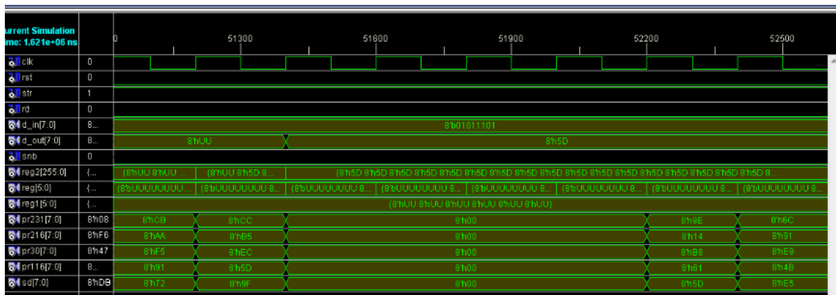
Figure 6.15; Test bench wave form of RS encoder
