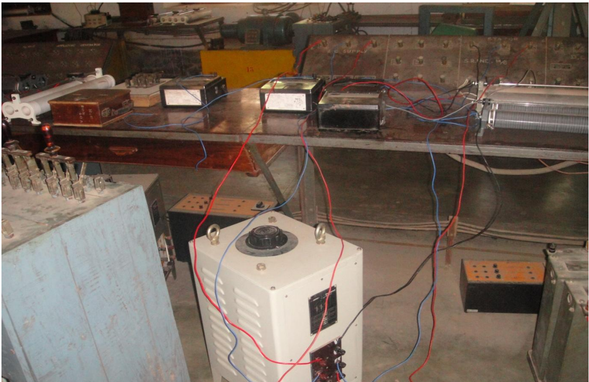
FIGURE 5.2: 3- \Phi Induction Machine coupled with DC motor
