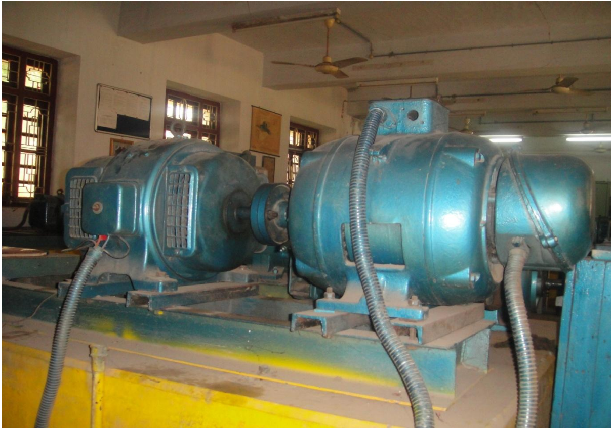
FIGURE 5.2: 3- \Phi Induction Machine coupled with DC motor
