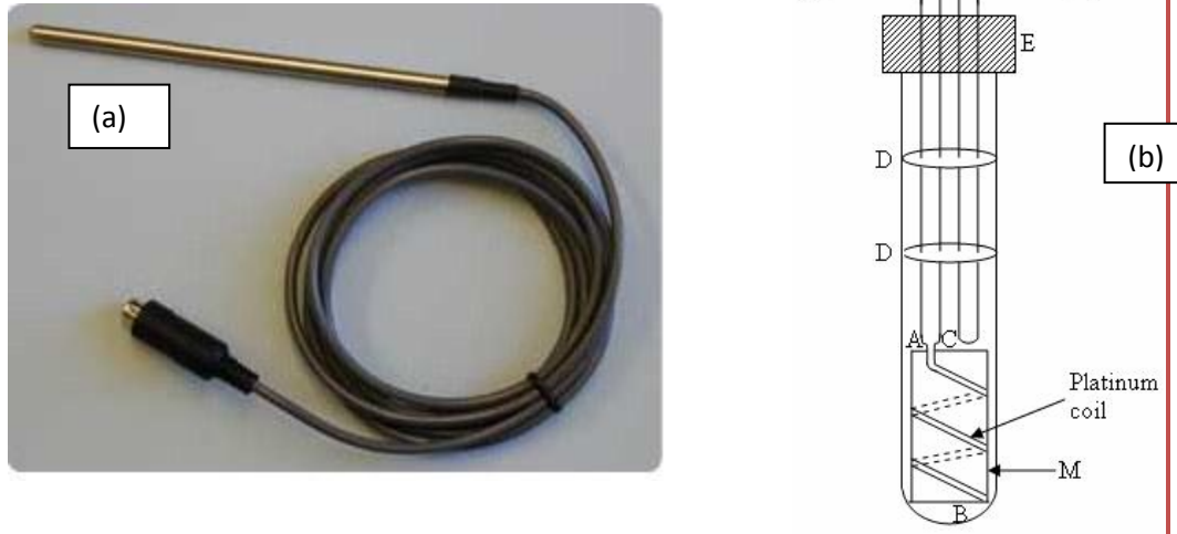
Fig 1.7 : Platinum resistance thermometer (a) Pt-100 probe (b) its schematic representation.[7]
