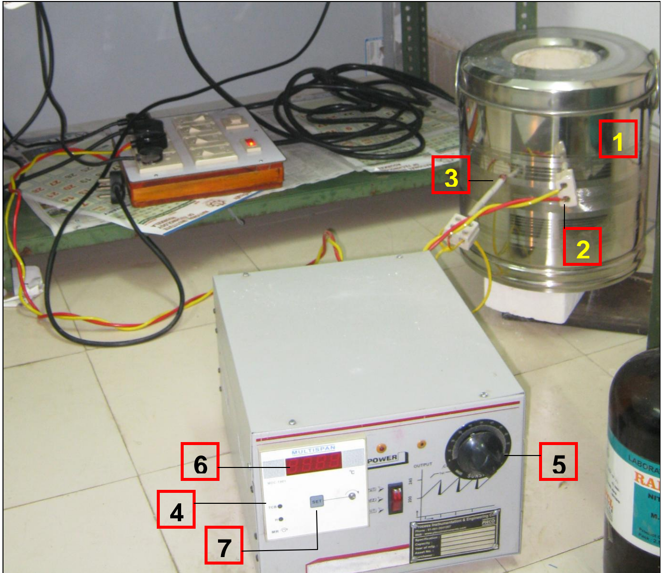
Fig 2.7: Furnace with temperature controller [1] Furnace; [2] Porcelain connectors for electrical connection; [3] thermocouple; [4] Temperature controller; [5] Power regulator; [6] Digital panel; [7] Set point adjust
