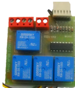
Figure 1.7: Skid Steer Relay Motor Driver
