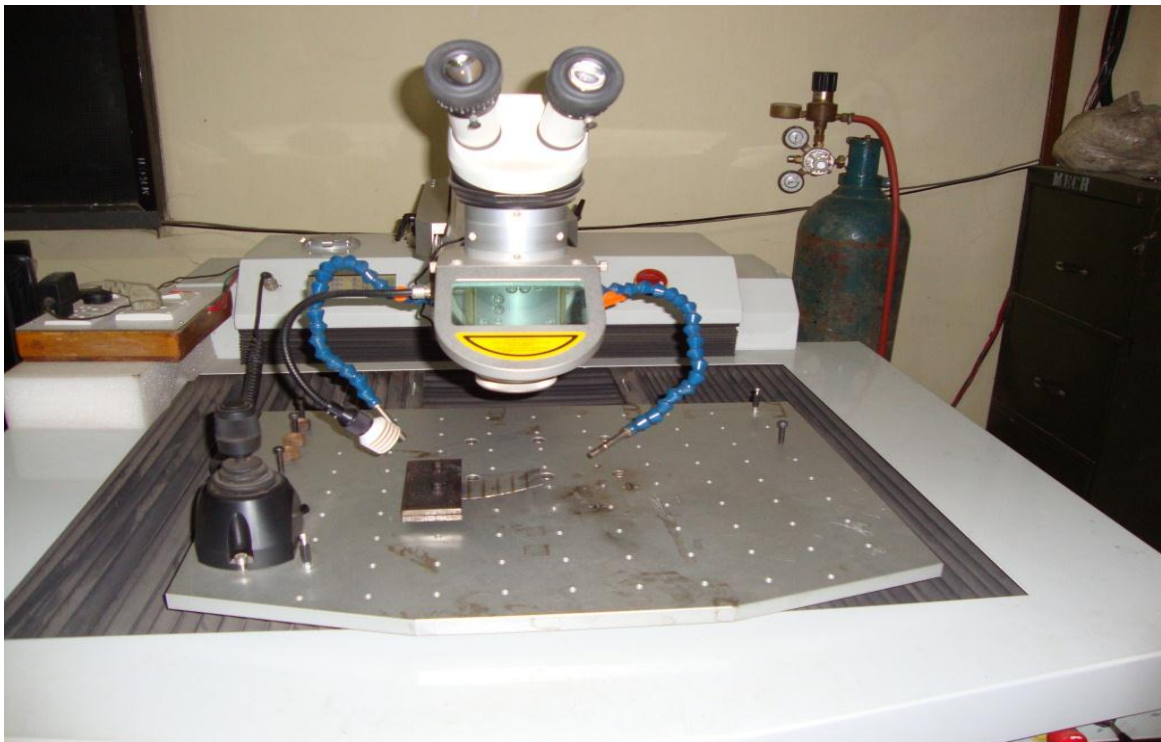
Fig : 3.2 Laser machine showing clamping and the work plate
