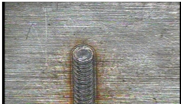
Fig: 3.4 w/p during laser beam scan
