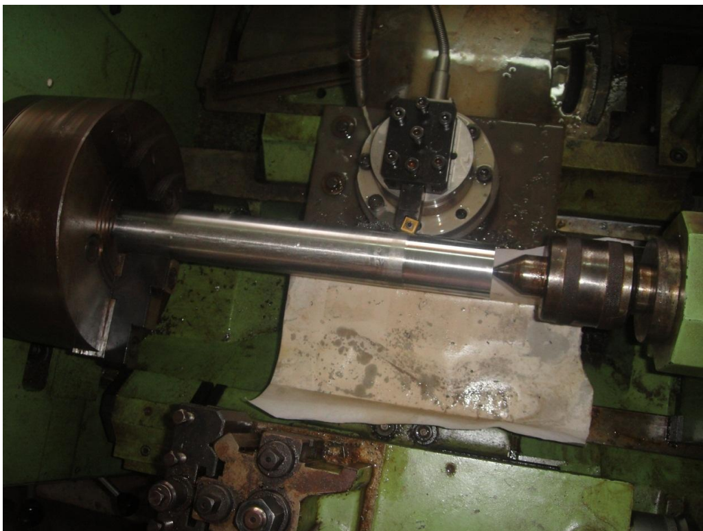
Fig a (attached W/P in chuck) Fig. b (tool, dynamometer and W/P assembly)
