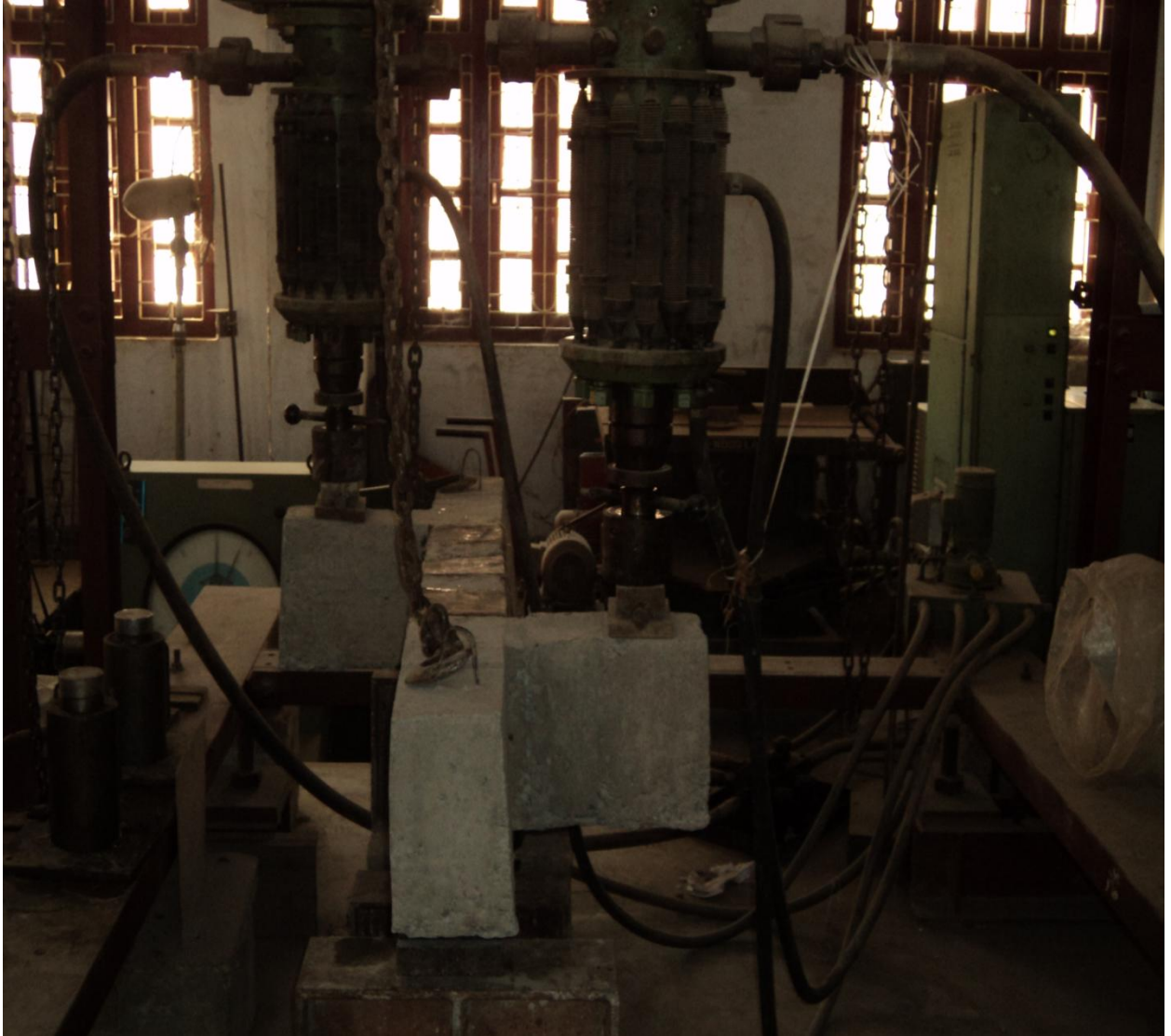
Fig. 7 Arrangement of the beam under the hydraulic Jacks
