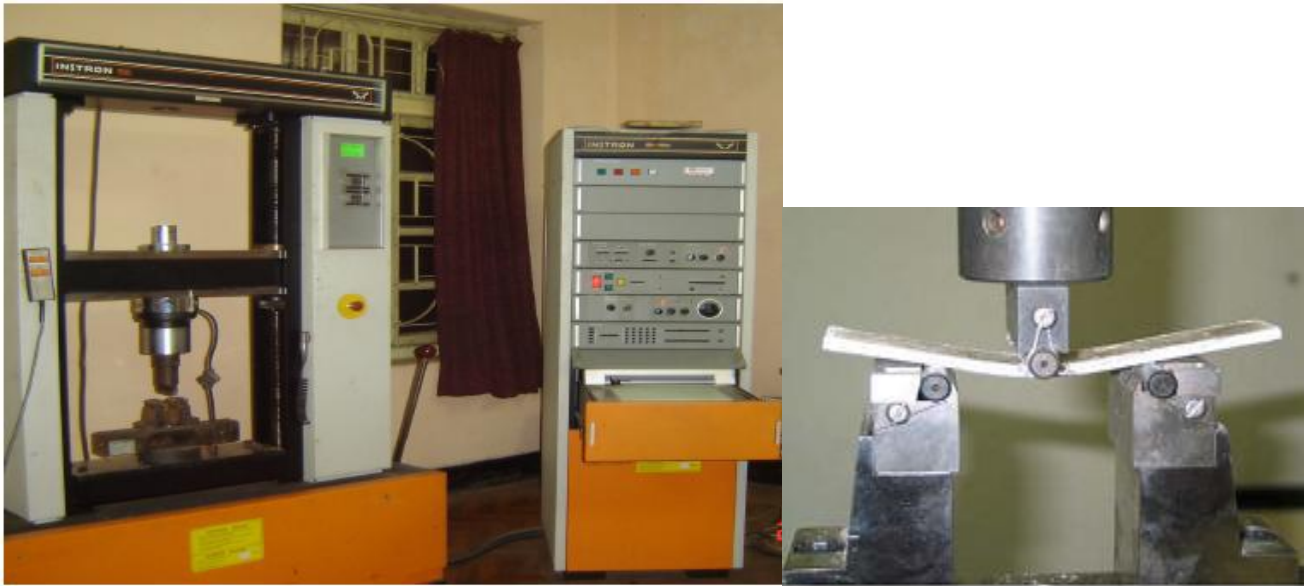
Fig 19 (a)-Instron 1195 with short beam shear test arrangement (b) Loading of sample and fracture during SBS Test
