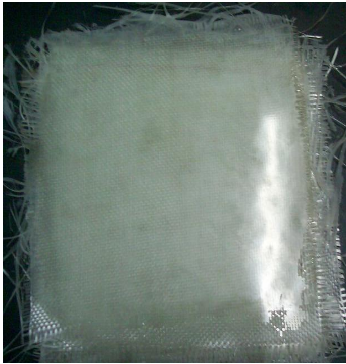
Fig 18-Glass fiber reinforced polymeric composite prepared by hand lay-up method
