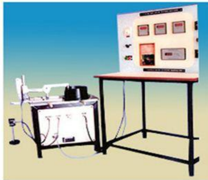
Fig. 2 Wear measuring test rig
