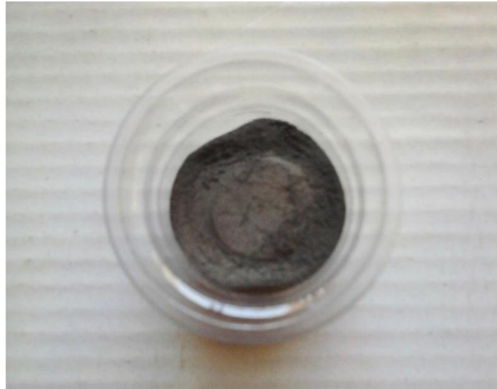
A picture of fly ash used in fabrication of fly ash - PEEK composite
