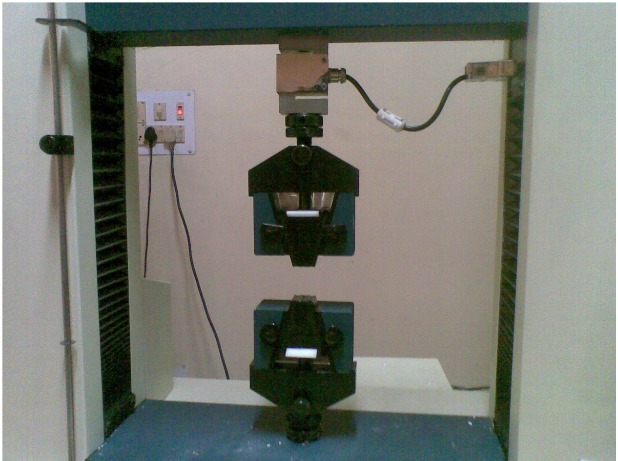
FIG(4.1) UTM machine Sample unloaded condition for tensile testing.
