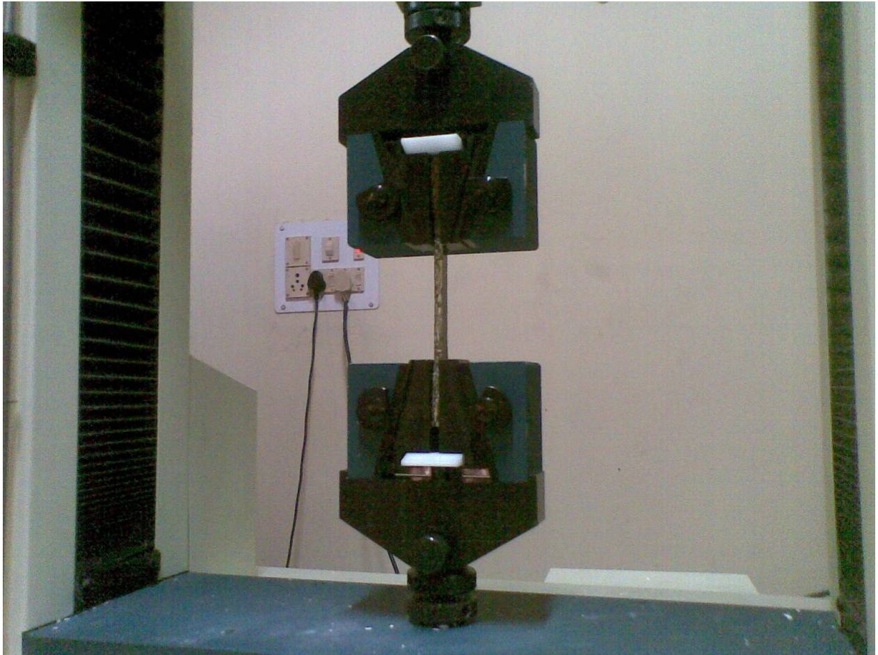
FIG(4.2) UTM machine Sample loaded condition for tensile testing.
