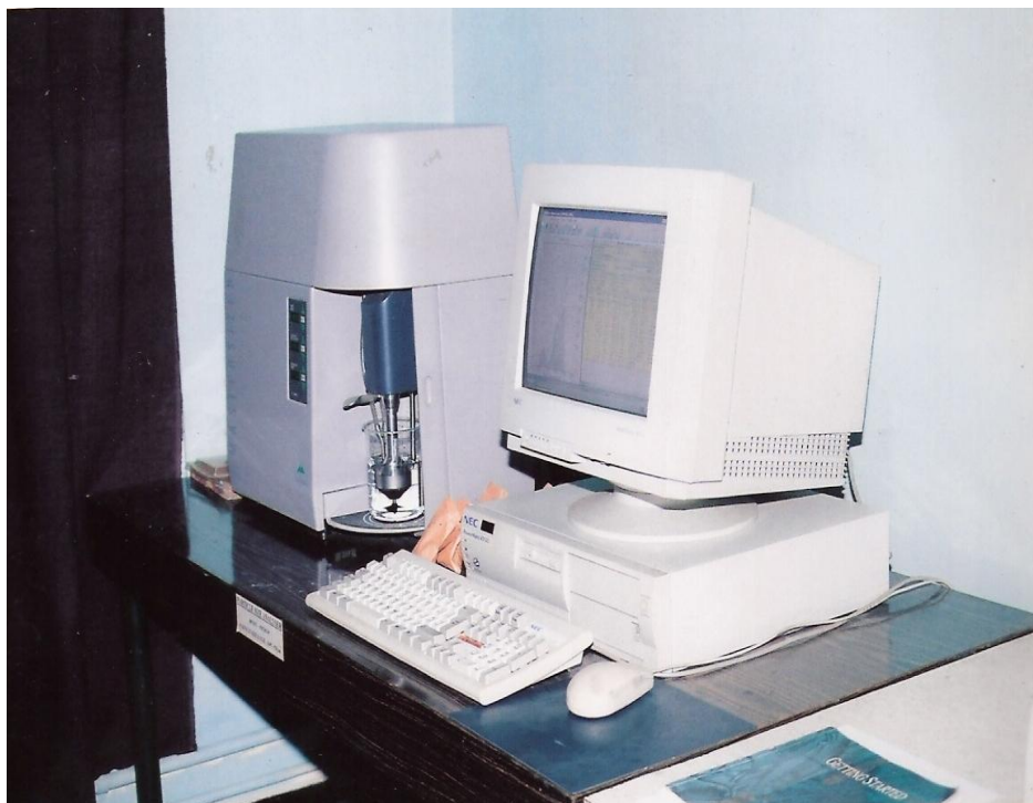
Fig.3.2 Malvern particle size analyzer (Model Micro-P, range 0.05-550 micron).
