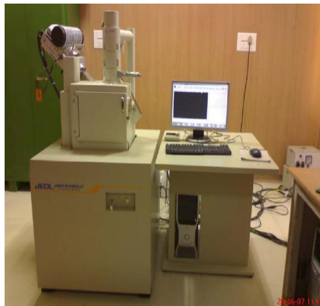
Fig.3.3 JEOL JSM-6480LV scanning electron microscope
