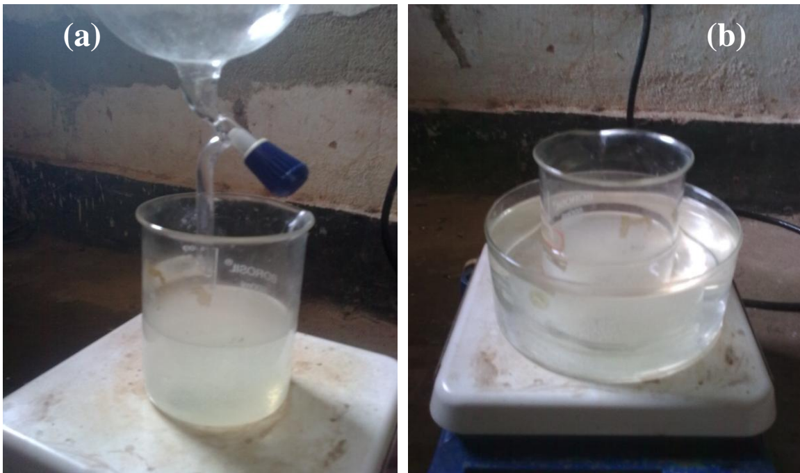
Fig. 2. Preparation of soda lime silica gel through sol-gel process; (a) addition of sodium silicate solution into calcium nitrate solution, (b) sol heated in hot water bath.
