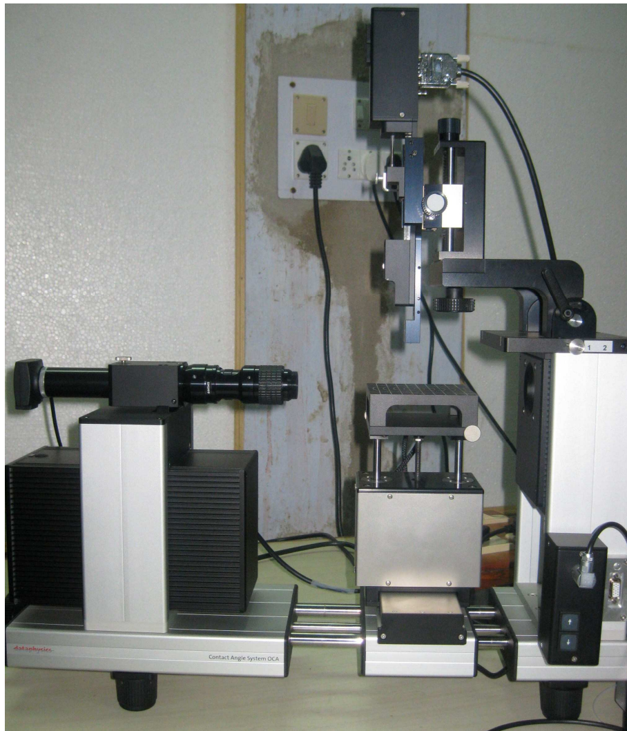
Figure-3.2: Photograph of video based optical contact angle meter
