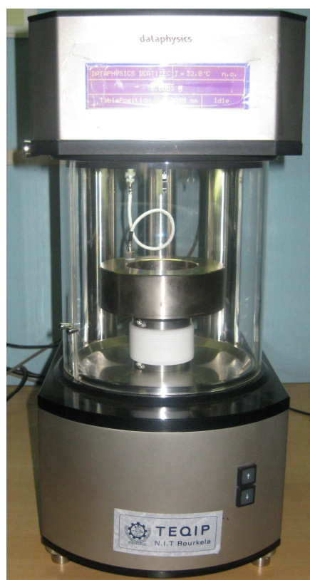
Figure-3.1: Photograph of Surface tensiometer
