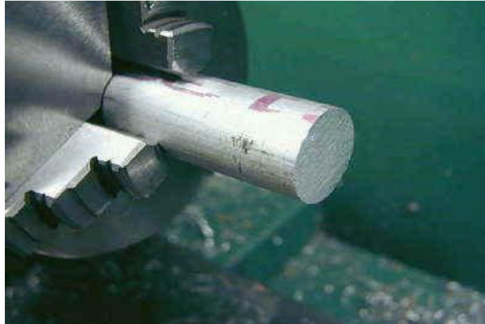
Figure 2: Work Piece Mounted On Chuck
