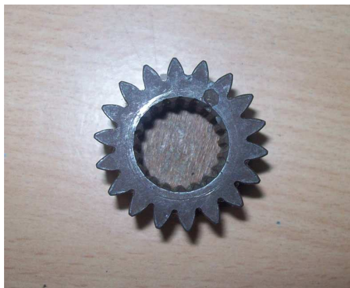
Central pinion (spur gear) attached to steering of AGV. Diameter of Pitch Circle=32mm
