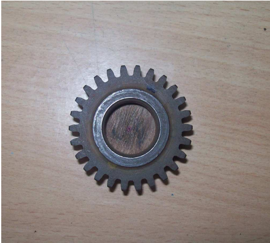
Pinion (spur Gear) that is attached to the servo motor for rotating the central pinion attached to the steering of vehicle. Diameter of pitch circle = 45mm
