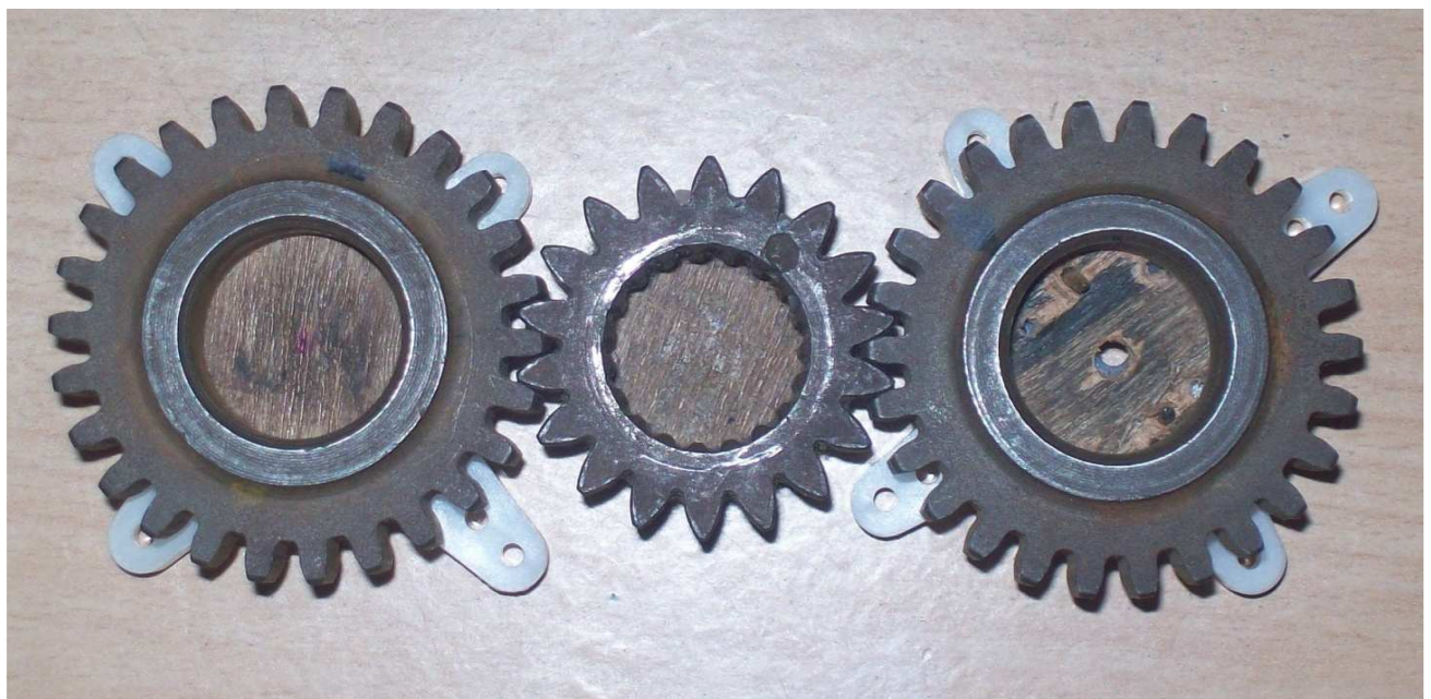
Dummy setup (as not affixed to steering handle) showing driving gears mating with driven.
