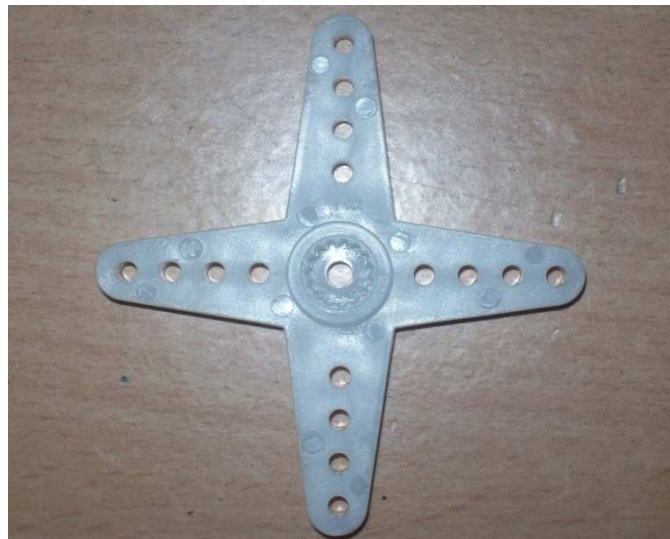
Arm Attached to servo shaft and permanently with the driving spur gears
