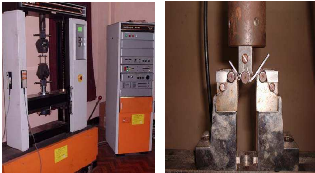
Figure 3.3 Experimental set up and loading arrangement for the specimens for tensile test and three points bend test.
