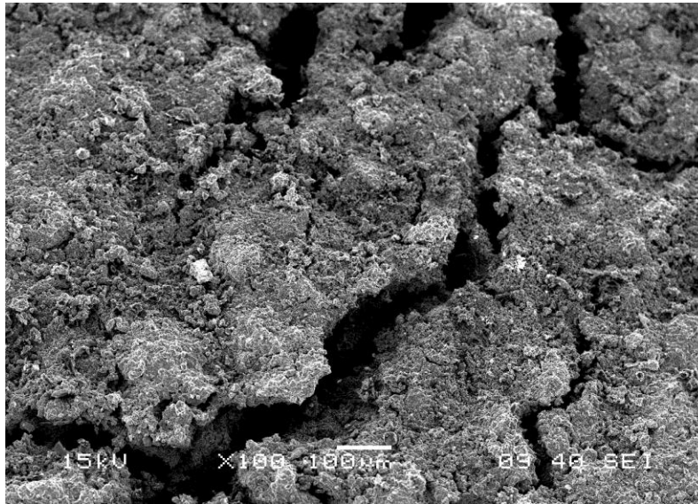
Fig: 4.11 SEM image of Sakaruddin iron ore pellet A type {-100# (100%)} reduced at temperature 950°C, Magnification 100X.
