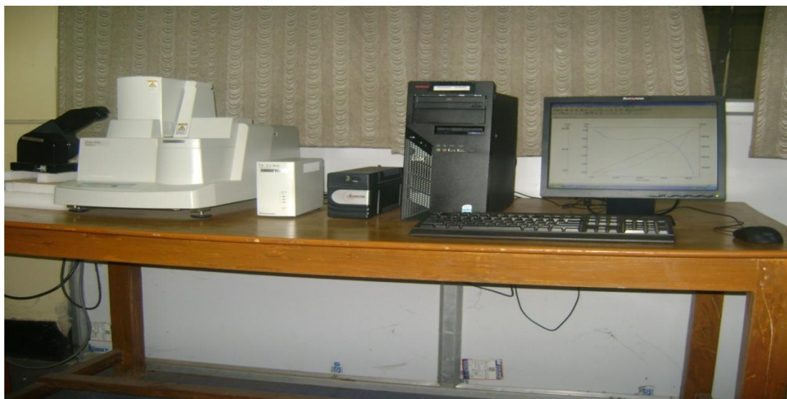
Fig 4.2: Experimental set up of differential thermal analysis
