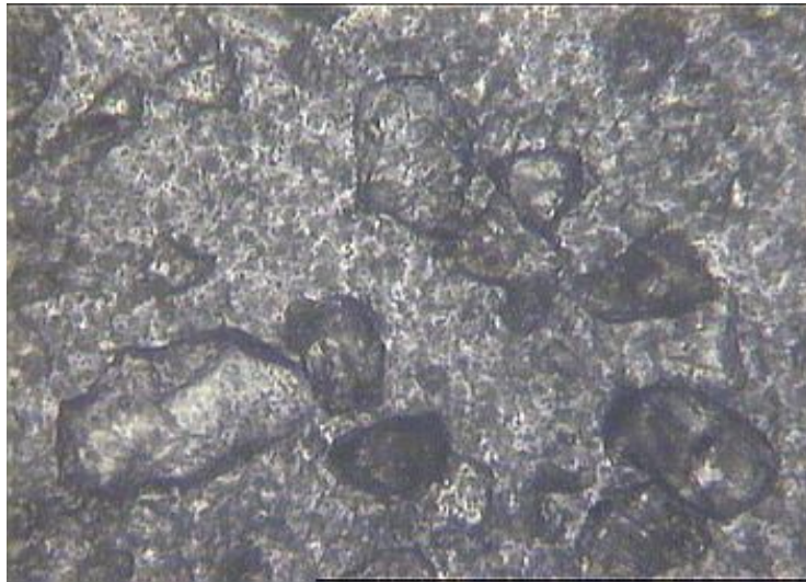
Fig. 14-SEM micrographs (magnification 100X) showing that the crystalline phase is Gehlenite
