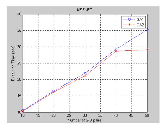
Fig.3: Simulation results on the performance of original algorithm and modified algorithm: Execution time of the Routing Vs Number of S-D node pairs in NSFNET.
