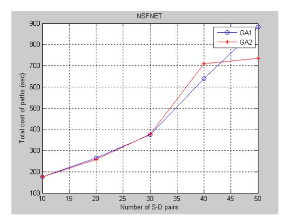
Fig.2: Simulation results on the performance of original algorithm and modified algorithm: Total cost of paths Vs Number of S-D node pairs (lightpath requests) in NSFNET.
