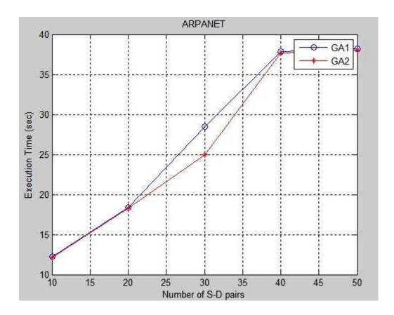
Fig.1: Simulation results on the performance of original algorithm and modified algorithm: Execution time of the routing Vs Number of S-D node pairs (lightpath requests) in ARPANET.
