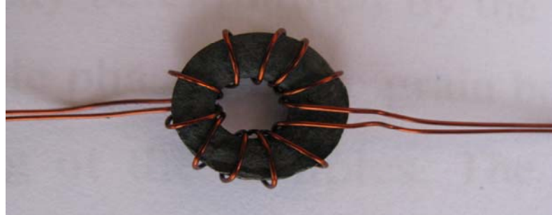
Fig. 3.5. Low capacitance winding of six turns on ferrite core.
