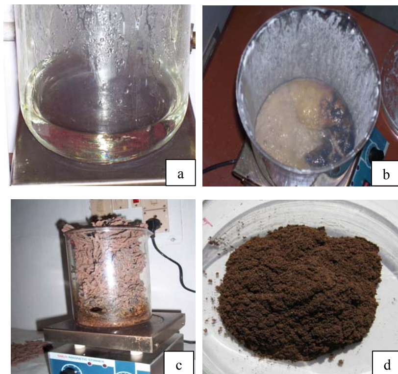
Fig. 3.2. Photograph of (a) nitrate-citrate solution, (b) dry gel, (c) auto combustion Reaction and (d) burnt ash powder.
