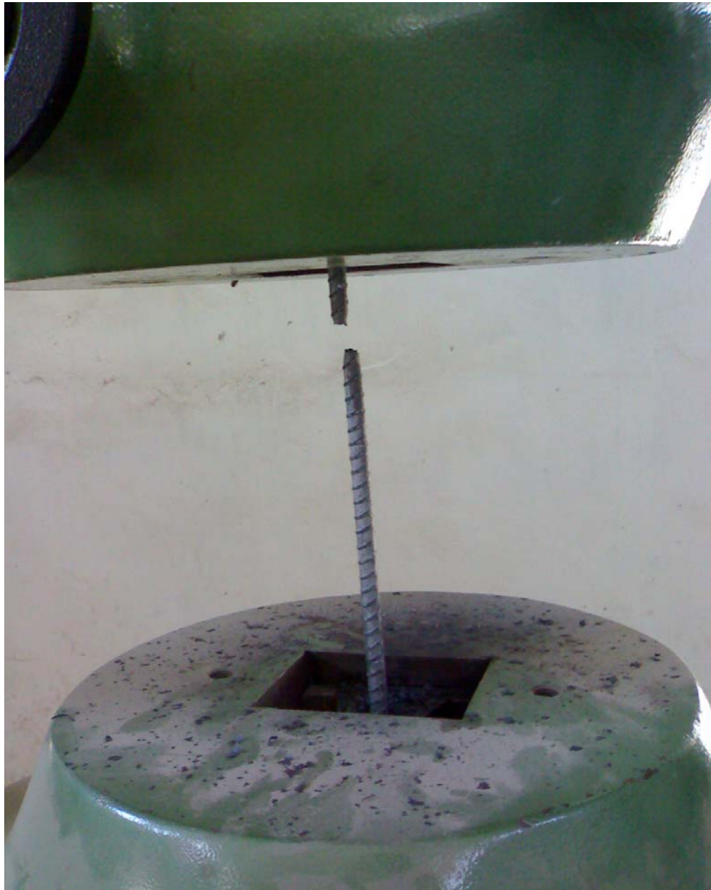
Specimen failed on UTM
