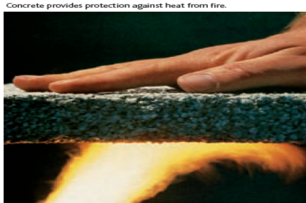
Fig1.3: Concrete against fire
