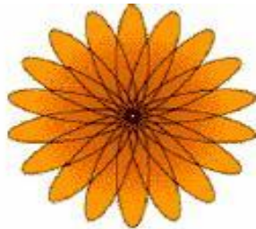
Fig.3.1. Switched Beam System Coverage Patterns
