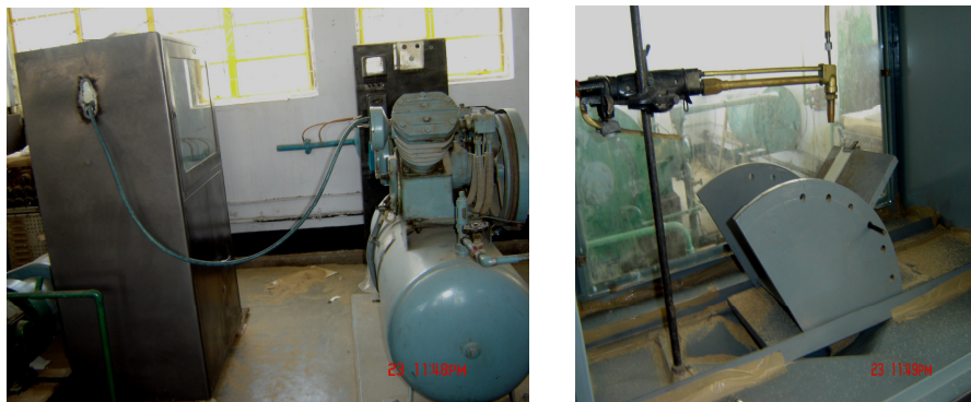
Figure 3.5 Solid Particle Erosion Test Set Up
