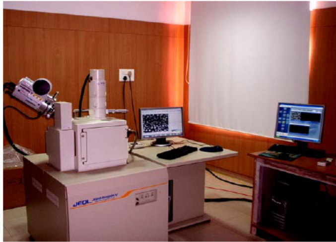
Figure 3.3 Scanning Electron Microscope JEOL JSM-6480LV
