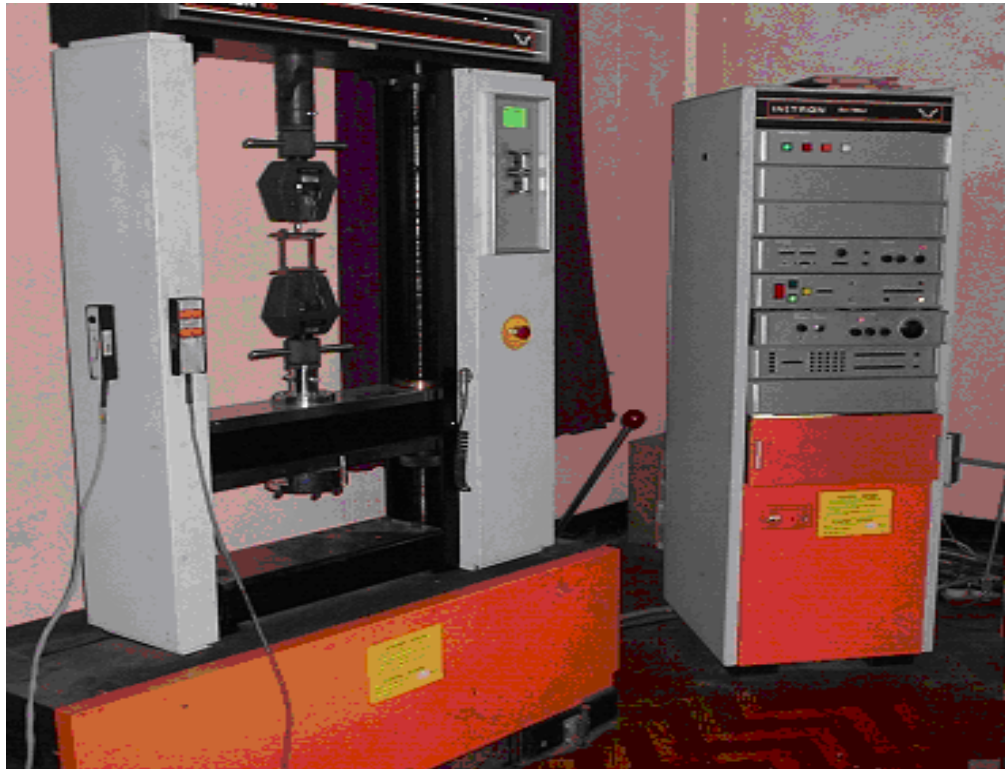
Fig. 3.5 Adhesion test set up Instron 1195
